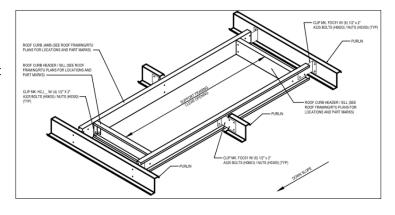
This will cause the adjacent, uncut purlins to be used to support both the RTU and loads from the cut purlins attached to the RTU jambs. This may require heavier purlins or even independent framing members to be used.
