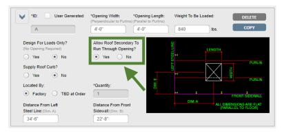
The first detail to look at is the weight of your RTU. NBS guidance requires that any RTU weighing more than 1,000 lbs. should have independent framing members. These members are usually built-up or hot rolled beams used to support the heavier RTU loads. This type of framing requires purlins to be cut, so there is little benefit for allowing purlins to run through the opening.
