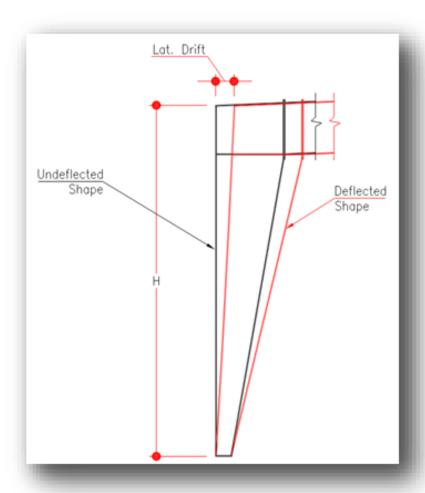
Figure 1 - Frame Lateral Drift (sidesway)
