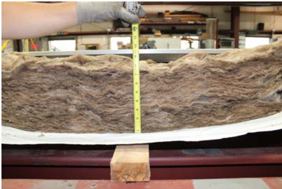
Proper Insulation at Mid Span (Fig.3)
