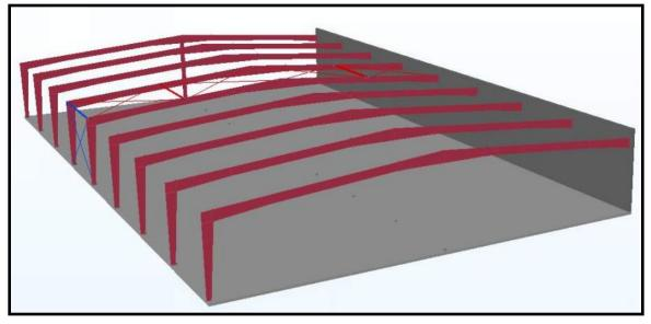
Shear walls are structural members, typically composed of pre-cast or tilt-up concrete wall panels, which are used to resist the building longitudinal forces.
