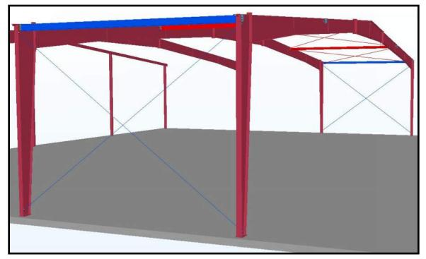
Full height X-Bracing is the standard Nucor Building System solution to longitudinal strength and stability and is the lowest cost option. The below guidelines are intended to provide guidance when utilizing full height X-Bracing.
