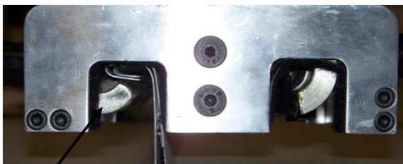
Stage One produces a "Vise Lock" Crimp
