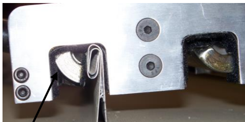
Stage Two produces a "Vise Lock 360" Crimp
