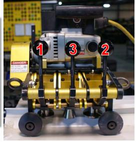
Insure that the center set of tooling rests on the "transition area" created by hand crimping while locking the machine onto the panel.
