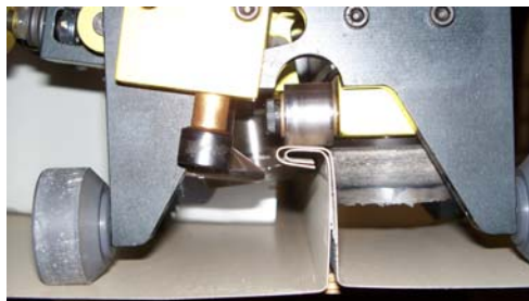
Seamer Locked on the Manually Crimped VR16 II panel
