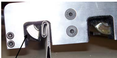
Stage Two produces a "Vise Lock 360" Crimp
