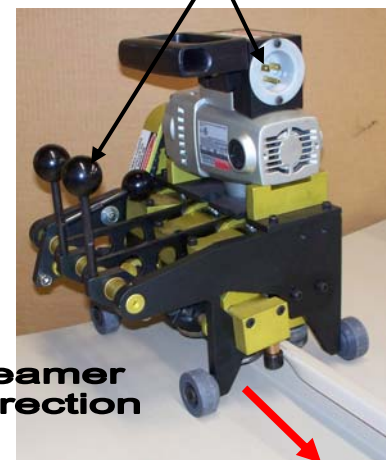
Seamer Locked on the Adjacent Seam
