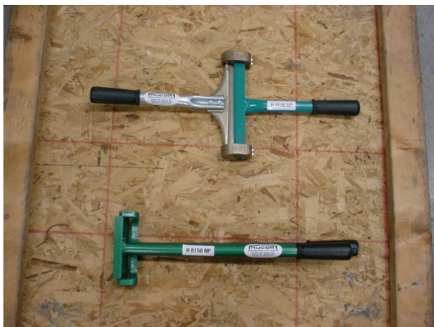
Small VL Hand Crimper H8100 (Top) Small VL360 Hand Crimper H8150 (Bottom)
