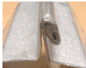
Finished “Nucor Vise Lock 360”™ Seam
